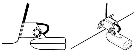
Route cable over bolt and through bracket. Side view shown (left) and seen from above (right).
